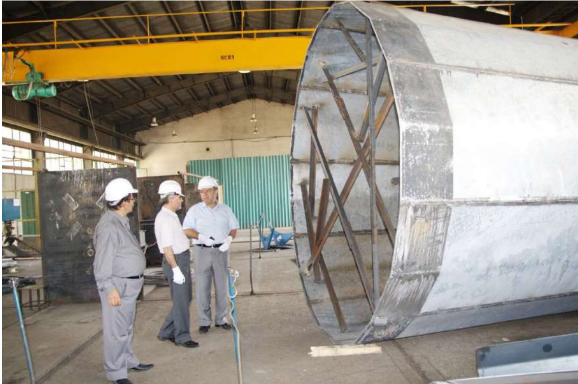
400 kv Poles for Fajr Petrochemical Co. under Manufacturing
